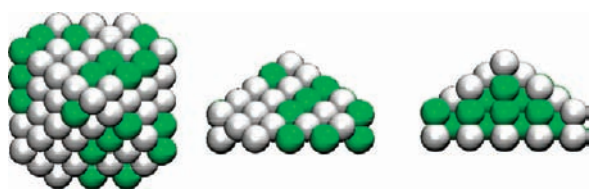
Figure 7. Schematic representation of a 110 atom, 1.7 nm Ir–Pt nanoparticle truncated by a (011) plane and possessing a hemispherical cuboctahedron morphology. From left to right, the images present views of the supported cluster viewed: perpendicular to the support, parallel to the support, and a cross section (to show the interior) of the cluster viewed parallel to the support. Pt atoms are depicted in white, and Ir atoms are shown in green.
